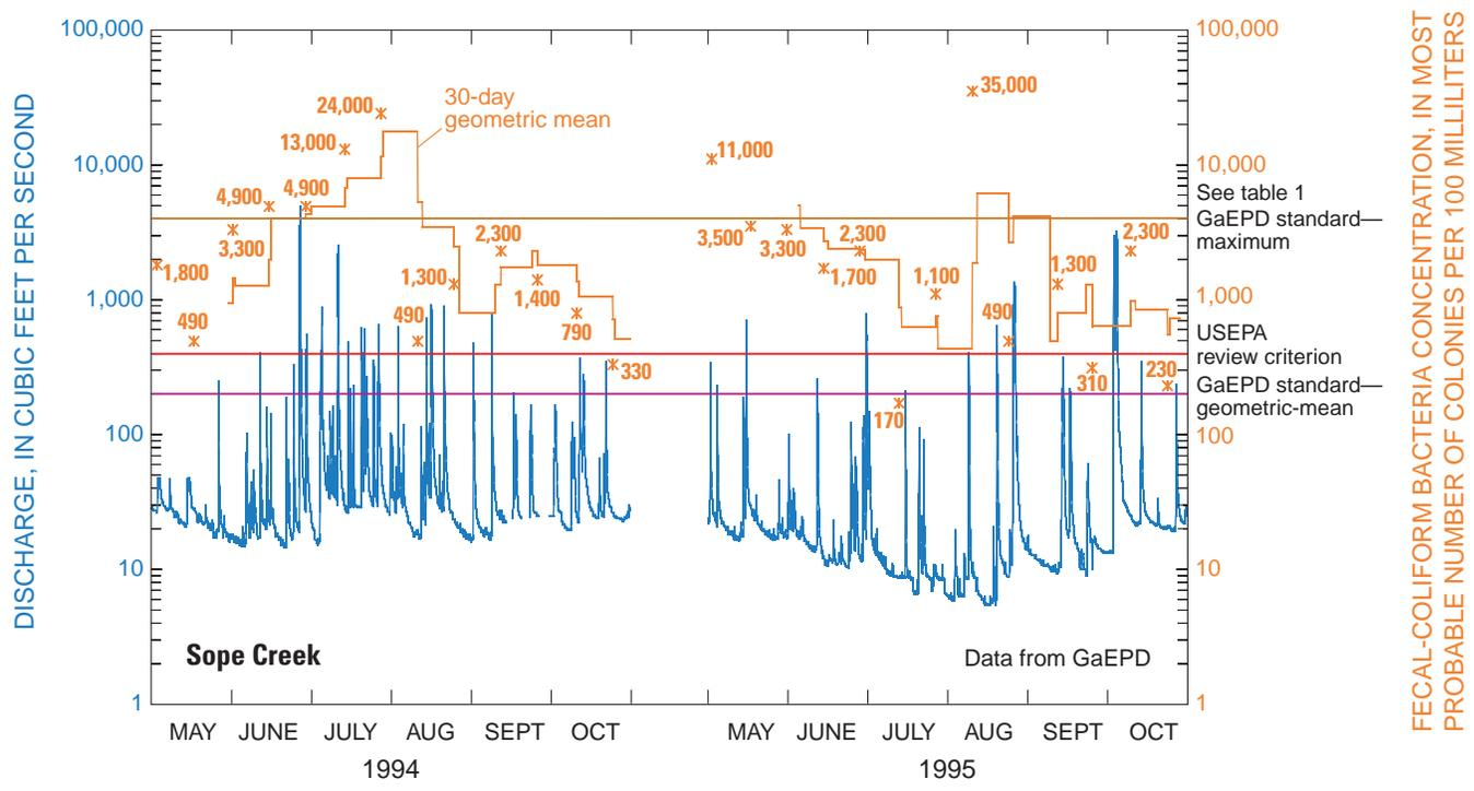
**Figure 4.** Stream discharge and fecal-coliform bacteria concentrations in Sope Creek, May–October 1994 and 1995. Concentrations of fecal-coliform bacteria in individual samples are denoted by an asterisk.
